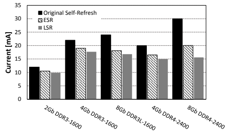
Figure 6: Comparison of current consumption between ESR, LSR, and original self-refresh modes calculated with Eq. 4.
